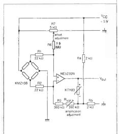
Simple drive circuitry incorporates temperature compensation
