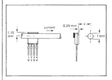
Measuring current. 1.5 mV/A measured with 2 mm separation from a 1 mm diameter wire, using a biasing magnet. This type of simple circuit lends itself for use as a non-precision ammeter or as an indicator for a burnt-out headlamp
