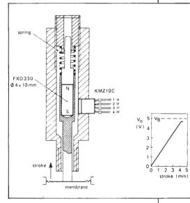
Pressure sensor. Membrane movement is transmitted to a permanent magnet. The magnet field is detected by the magnetoresistive sensor. The smaller diagram shows the displacement/voltage characteristic of an amplified, compensated output
